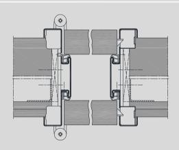
Version with flush closing door leaf, illustration for stud and brick walls.
